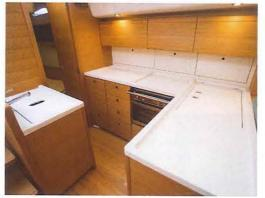
Galley The offset companionway helps to create space for a practically laid-out galley. The inboard island incorporating the sink provides useful support for working at heel and the generous work surfaces have high fiddles. There is plenty of stowage in the galley area in the form of soft-closing drawers, deep, raised lockers (which continue through the saloon), bottle stowage in the bilges and a bin area below the sinks.
