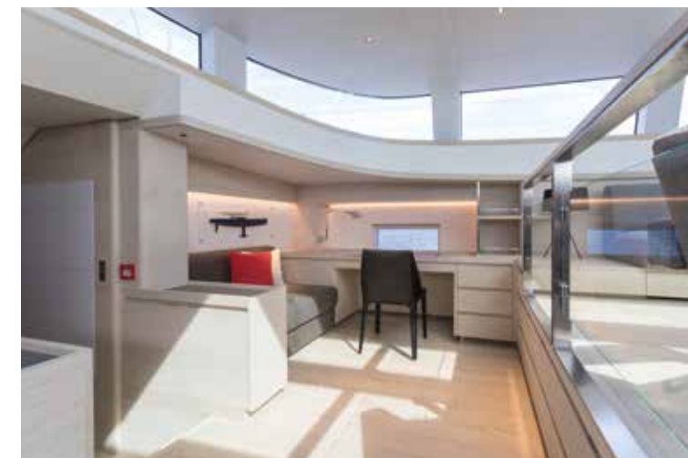
A glass balustrade with drawers underneath for storing serveware and an enlarged portlight facing the desk have opened up the lower saloon's office area
