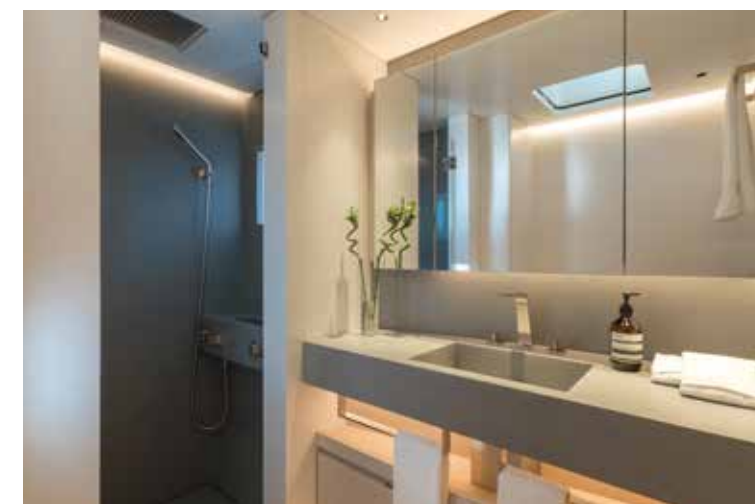
The lighting design for the en suites, with wall washer lights in the showers and rope lighting to illuminate faces at the basin, was presented in a full mock-up before installation
